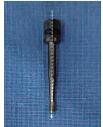
Fig. 5. When using a manual tool such as the Screw Removal Tip, not using the guide is recommended because the guide forces the one direction rotation when the tool needs to perform a random rotation. In fact, when trying to remove the fragments that could not be removed with a drill, the hole is not aligned with the actual axis of the implant orientation.
